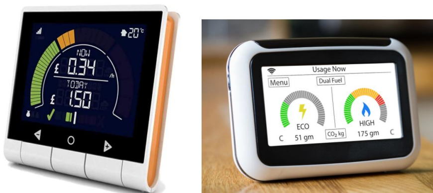
Figure 3.1 Example of Smart Energy Display Devices
