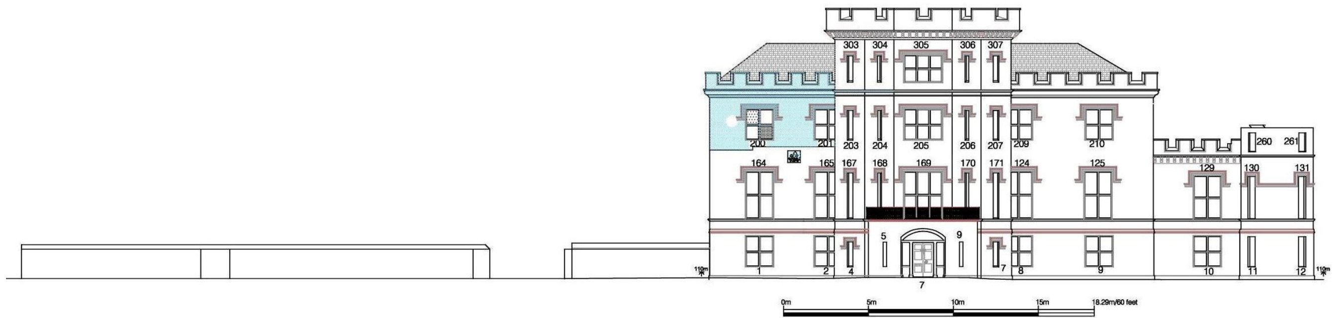
Fig. 33. Top: the East facade as built and as-existing (uncoloured), with the c.1892 raising of the South Wing shown shaded. Below: Paterson's 1801 design for the 'East or Entrance Front' showing the symmetry of the original design and the present courtyard wall on the site of Paterson's un-realised Stable Court. The scale to which Paterson's ambitious design over-reached Francis Sitwell's finances is obvious, as is the narrowness of the proposed Gatehouse compared with that as-built. There appears to have been a proposed heraldic device – a shield and swags – on the Gatehouse roof parapet.
