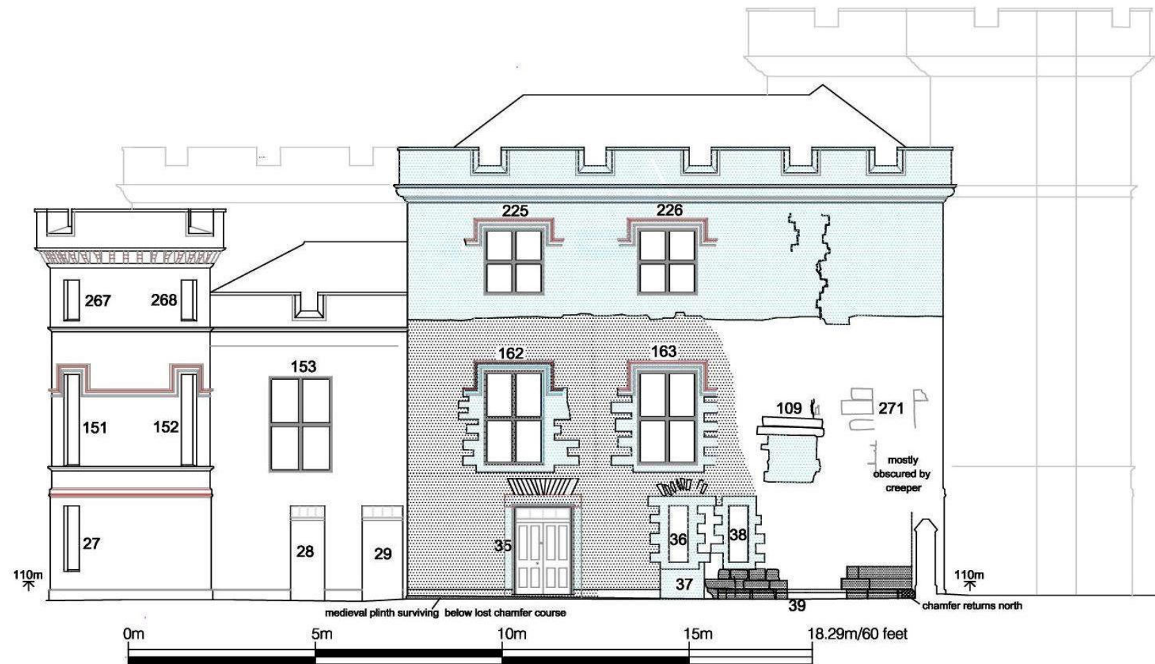
Fig. 36. Top: south elevation as built and as-existing, with the c.1892 raising of the South Wing, and associated alterations shown with blue shading. Surviving medieval fabric (where identifiable) is shaded black, and the possible late 18 th century remodelling, the extent of which is not clearly definable, in grey. The 1801-4 build is uncoloured, and includes features intended to serve the unbuilt 'Study' and 'Family Bedroom'. Below: Paterson's 1801 proposed 'South Profile' with the unbuilt extension to the east facade obscuring most of the South Wing.
