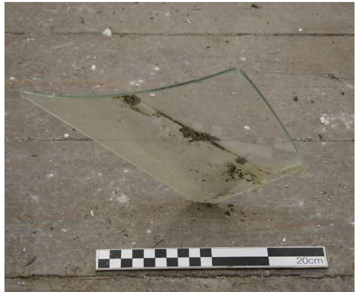
P124. R41, the glazed cupola over the Oval Saloon. Some minor delapidations since 2012 are apparent, largely a result of Storm Arwen which resulted in the shard of glass embedded in the floorboards
