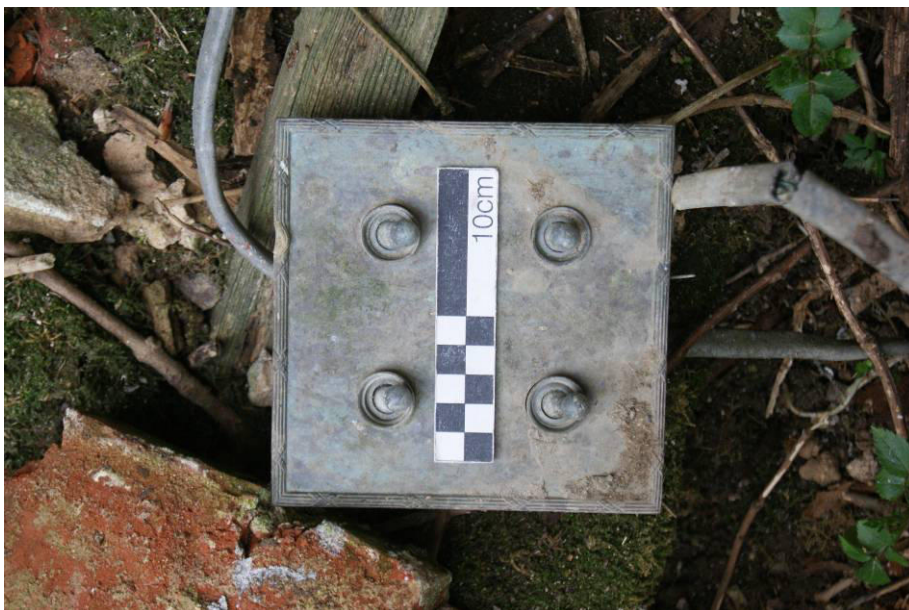
P90. North Range. R22. Detached 1923 light switch with 'Tucker Telac' insulators lying in the debris.
