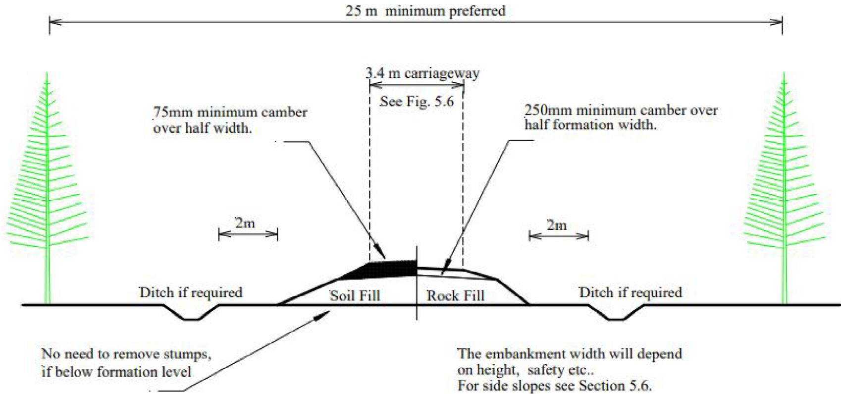
**Figure 5.2 Embankment on Good Foundation**
