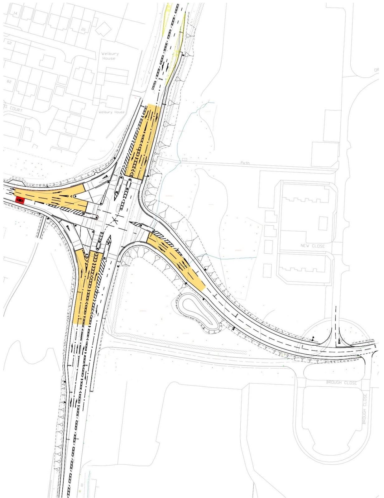
Figure 5A - Highway and Road Markings Design Layout
