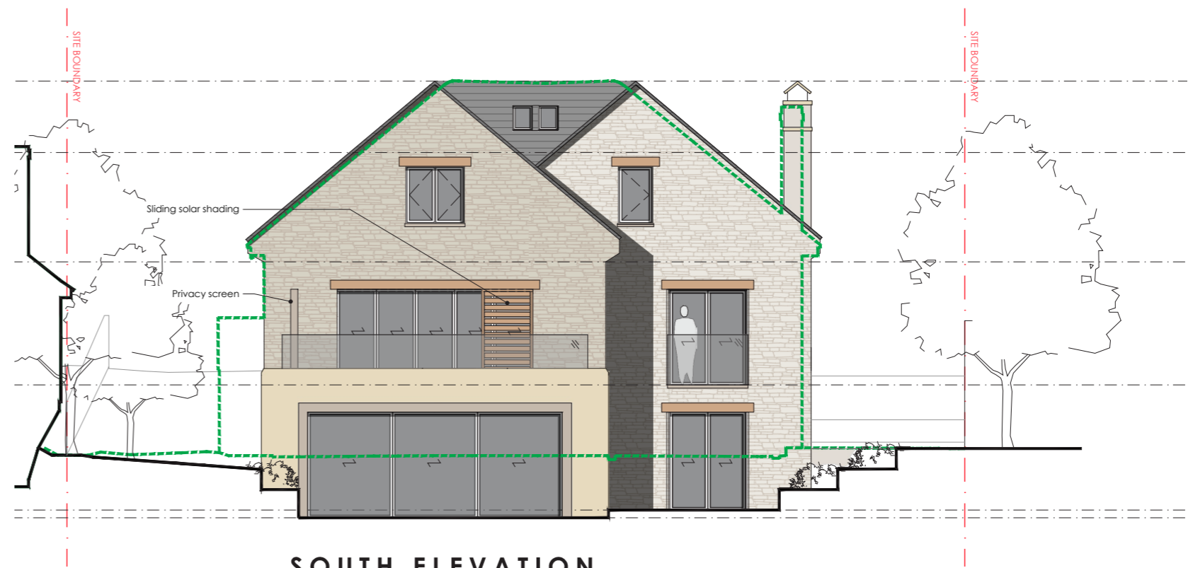
SOUTH ELEVATION Proposed south elevation is built further into ground. Topo to east and west to remain similar to existing
