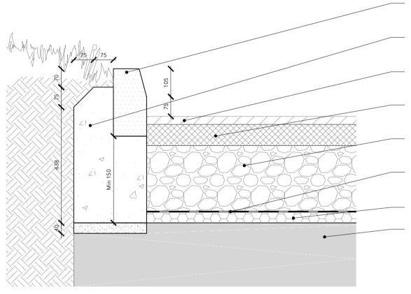
Proprietary HB2 Pre-Cast Concrete Kerb upstand to meet BS EN 1340
