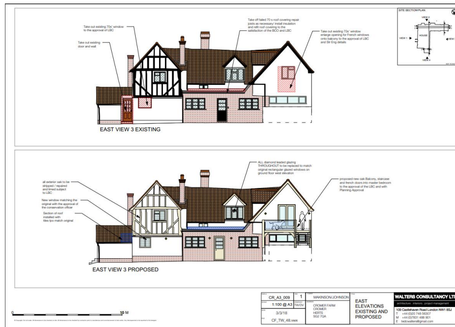
Figure 1 Existing and proposed east elevation extract from 2018 approved plans
