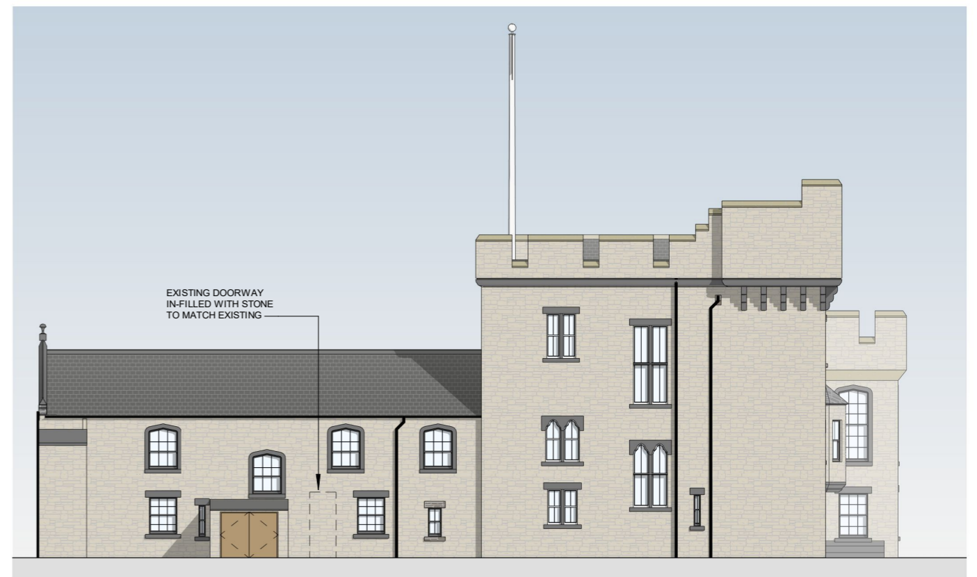
PROPOSED WEST ELEVATION SCALE 1 : 200
