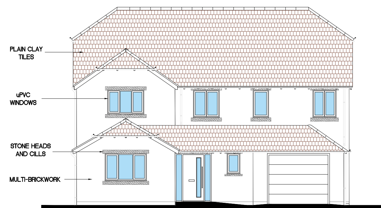
NORTH-WEST ELEVATION (FRONT)
