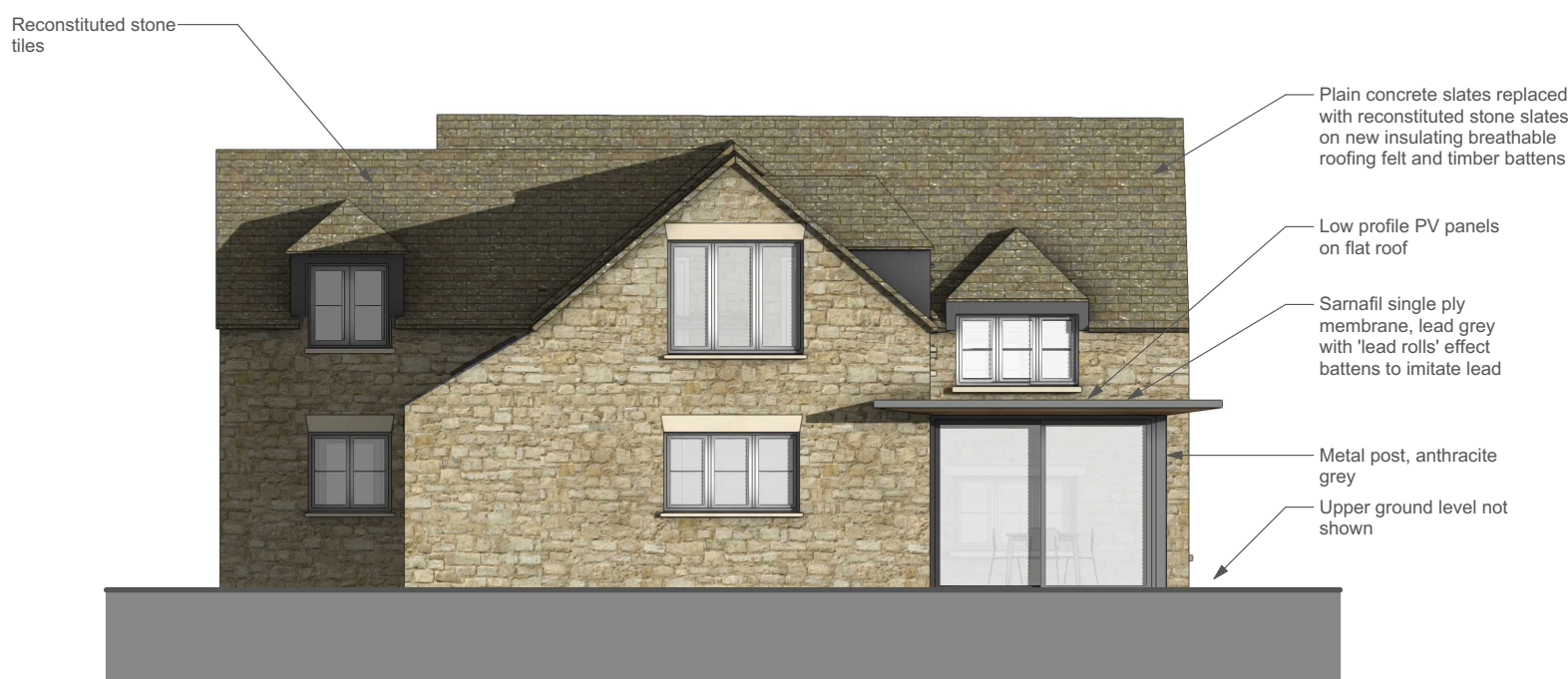
NORTH WEST ELEVATION
