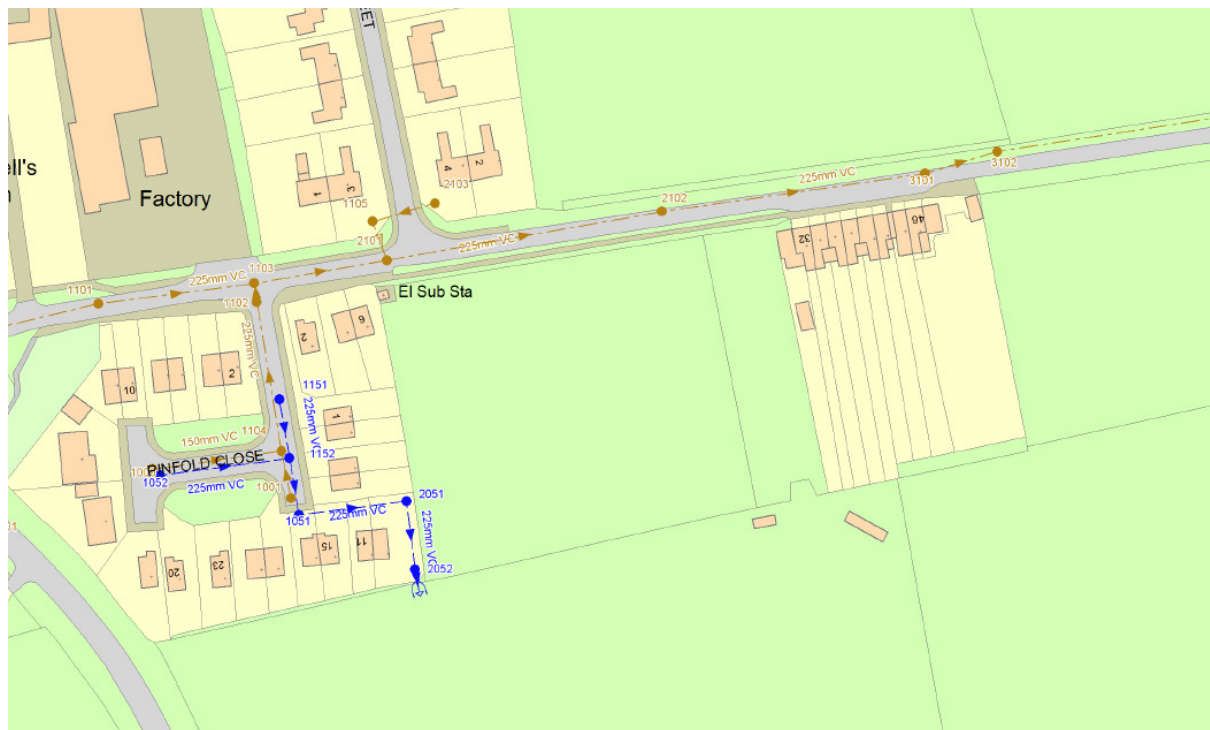
Figure 14 - Foul Connection into The Drive
