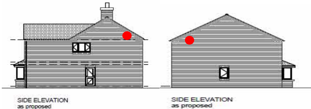
Figure 8.3 - (L) Location of integrated bat box on Plots 1 and 18 west elevation (R) – Location of integrated bat box on Plots 11 and 13 West gable ends.
