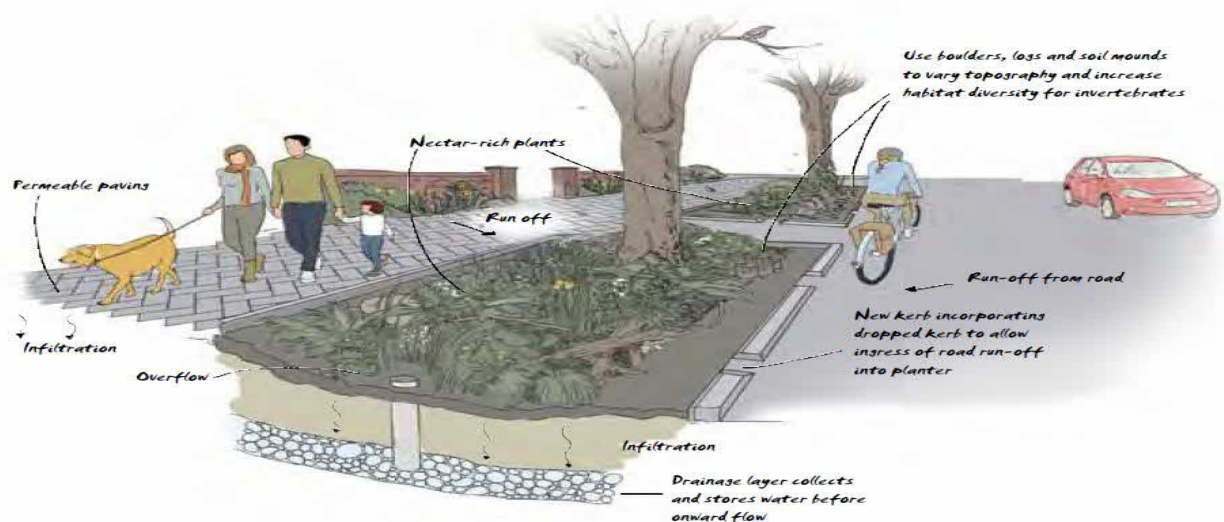
Figure 8.2 – Diagram illustrating dropped kerbs to allow surface run-off 33
