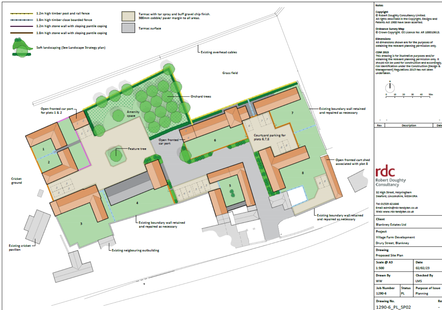
DWG no 1290-6-PL-SP02 showing proposed site plan with landscaping and boundary treatments. Open cart sheds (building C on 1290-6-PL-SP01 is not converted but retained as part of Plot 8.
