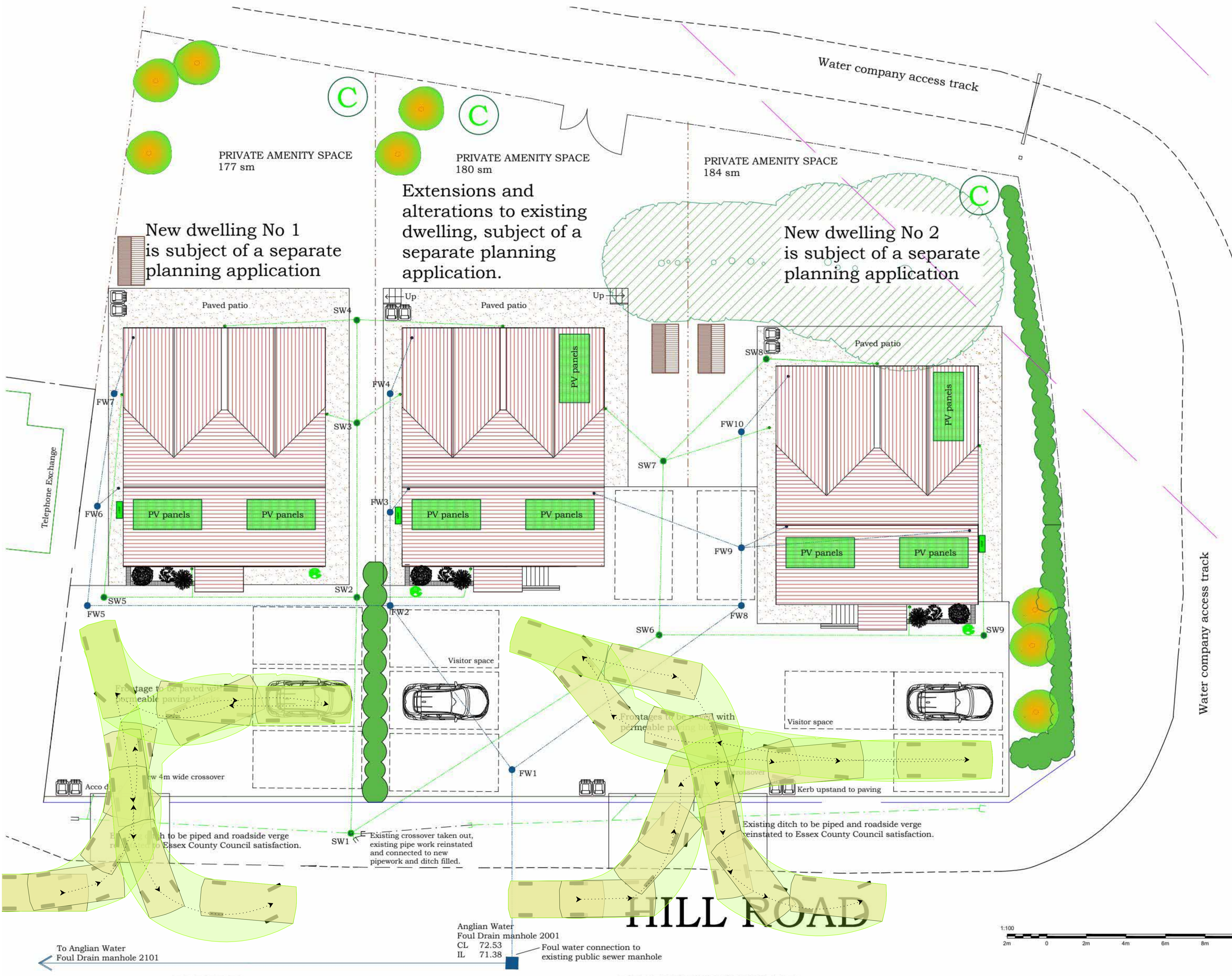
Residential development at 6 Hill Road, Gt Sampford CB10 2RT Proposed master site layout Drawing No RMDS/HR/2002 Scale 1:100 @ A1
