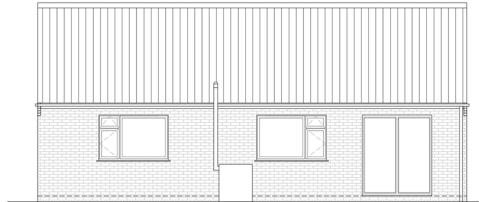
Proposed Rear Elevation (As Existing)
