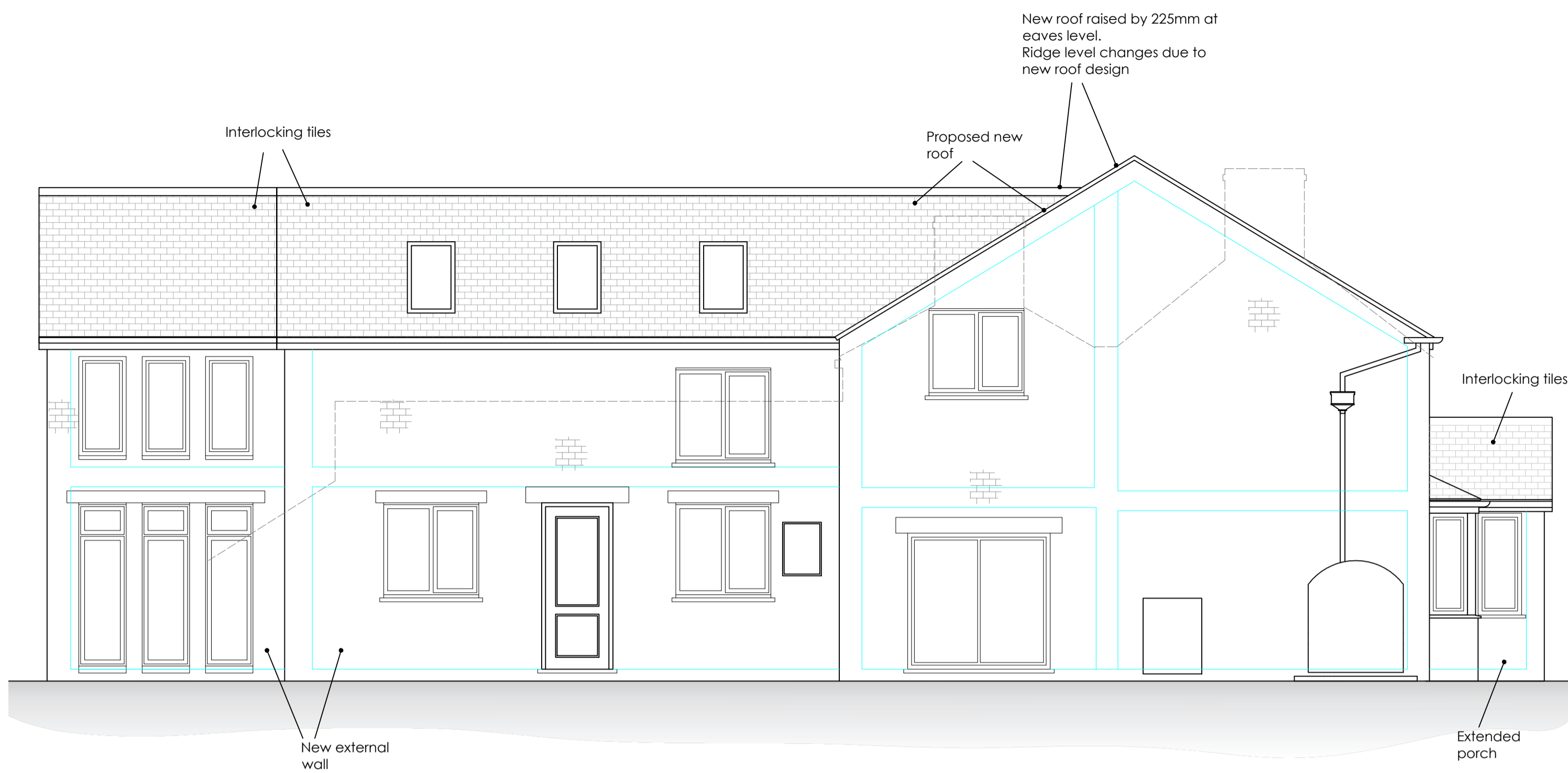
PROPOSED WEST ELEVATION 1:50
