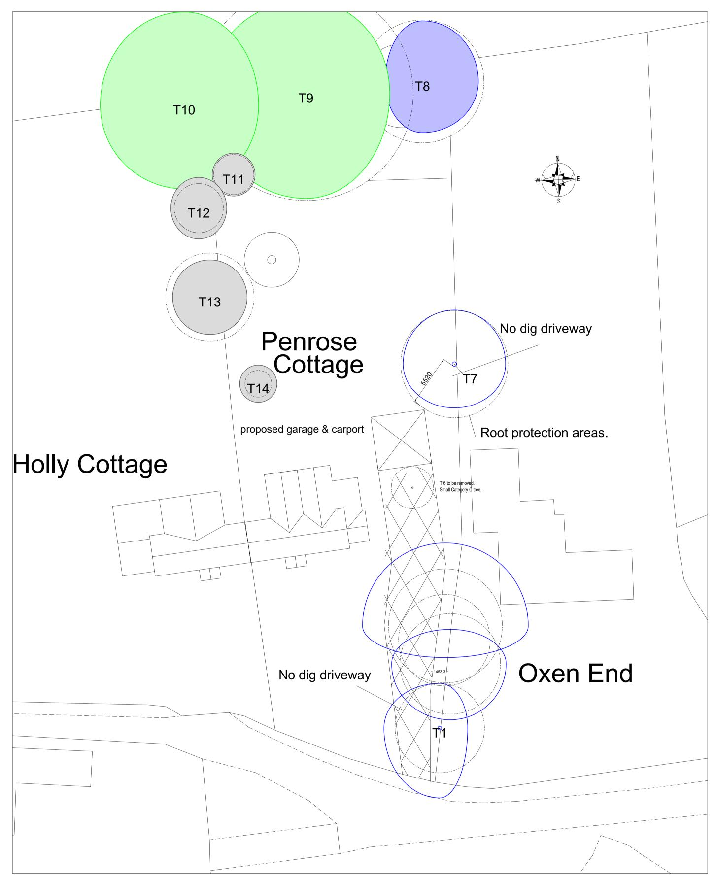
Through Access to maintain 500mm Distance from boundary and be minimum 3000mm Wide. Garage/ carport slab to be laid where illustrated. Scaled plan of garage/ carport on seperate drawing. No dig driveway 5 meters before and after centre of marked tree in order to protect roots.
