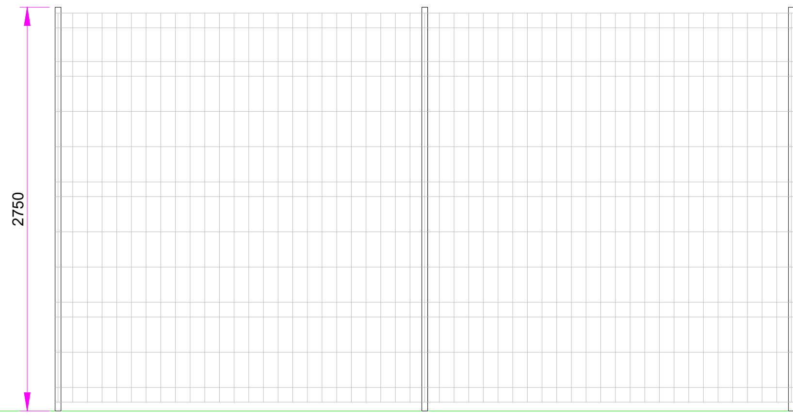
WELDED MESH FENCE ELEVATION
