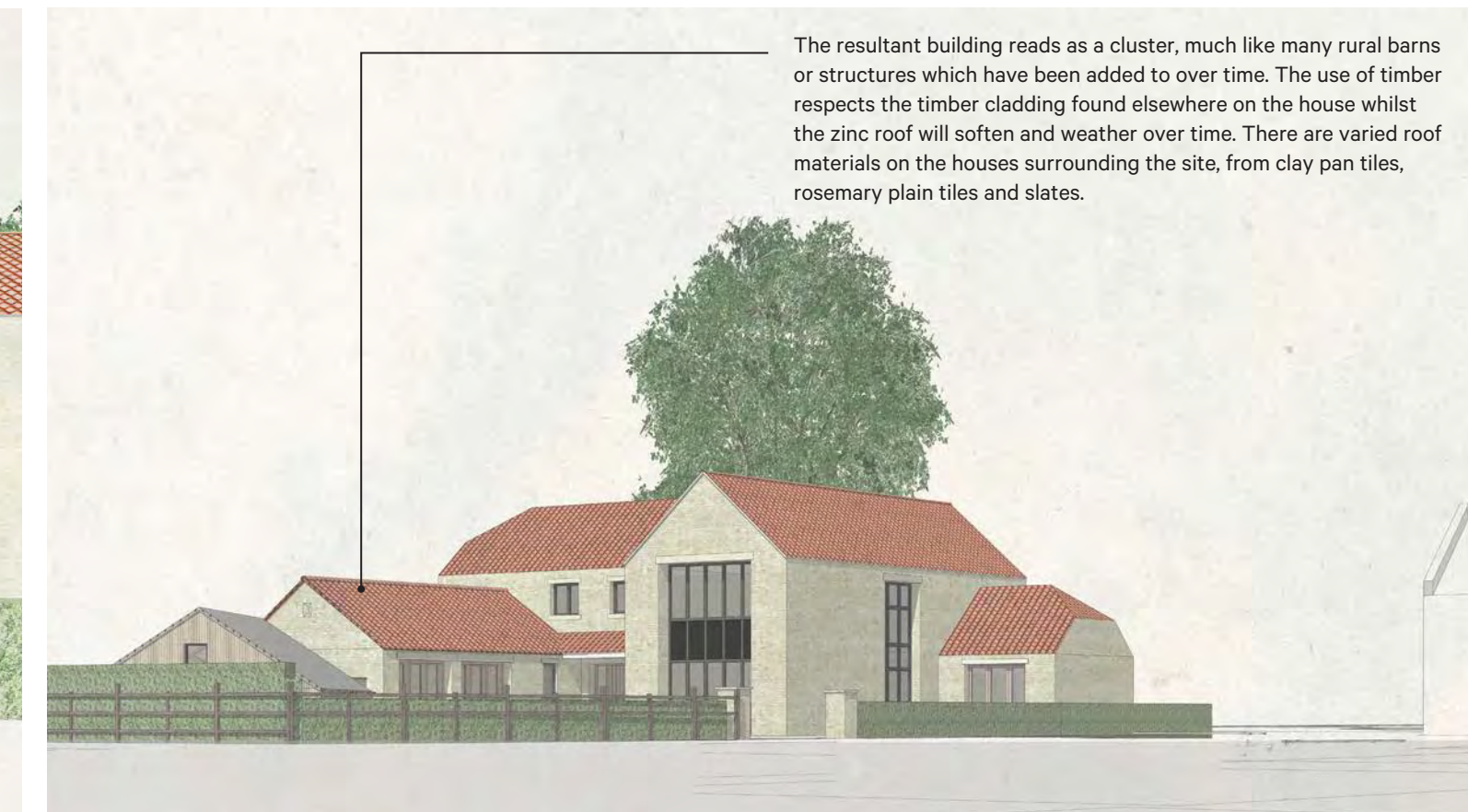
Illustration of the completed massing, with various roof forms and articulated wings. Note the lower ridge height of the proposed garage.
