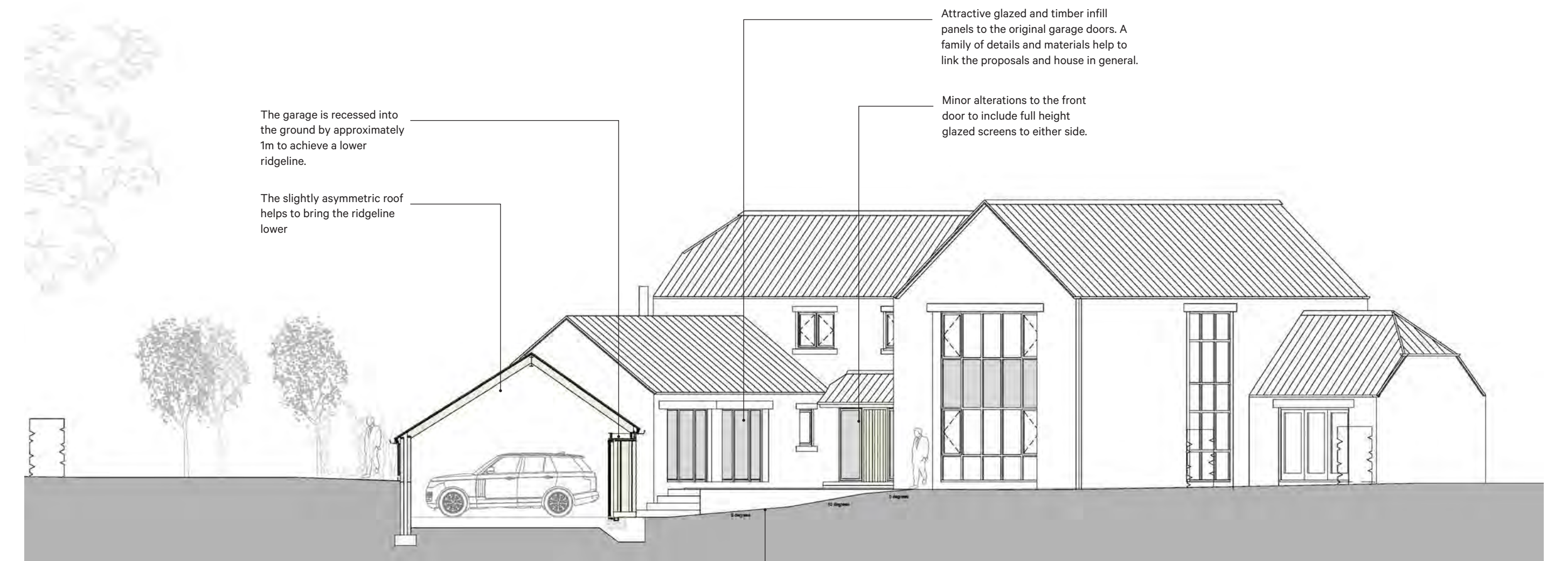
Proposed south-east elevation and section through garage
