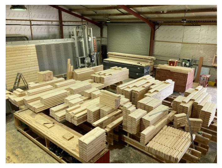
All components have identity markings corresponding to the installation plans, providing the manufacturing operatives the information required to assemble the mobile home or twin unit caravan.
