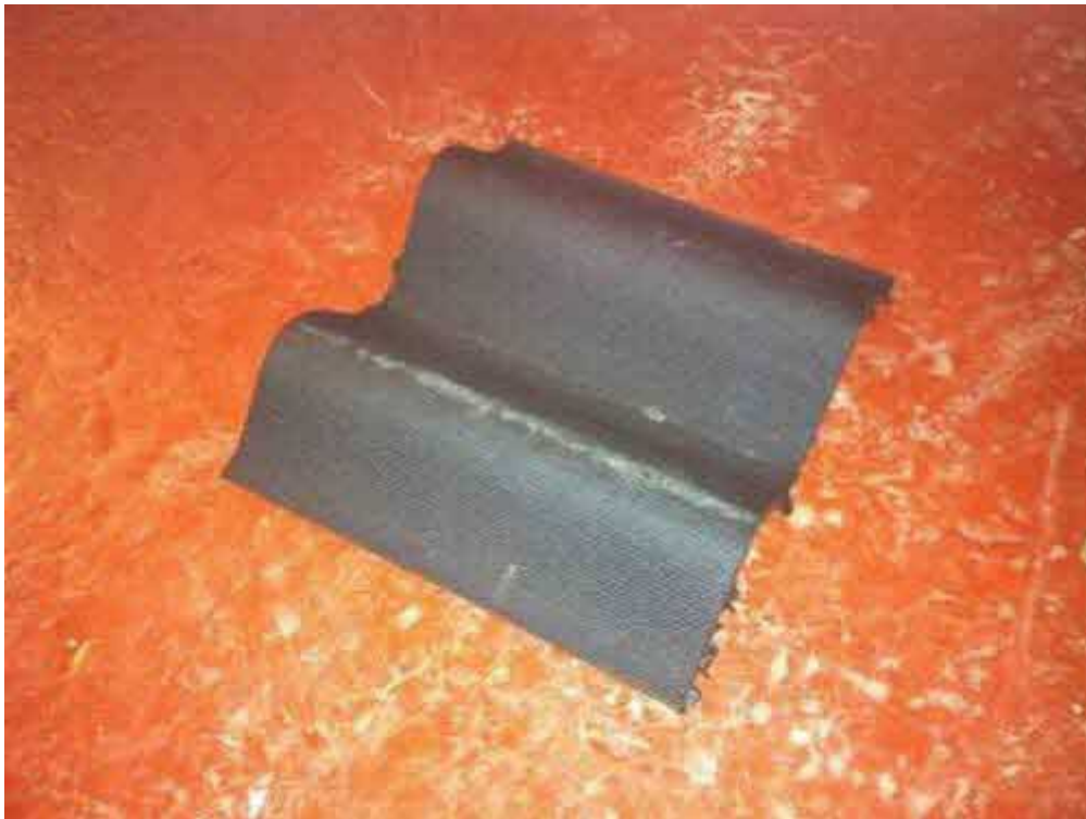
Typical example of corrugated roof sheeting
