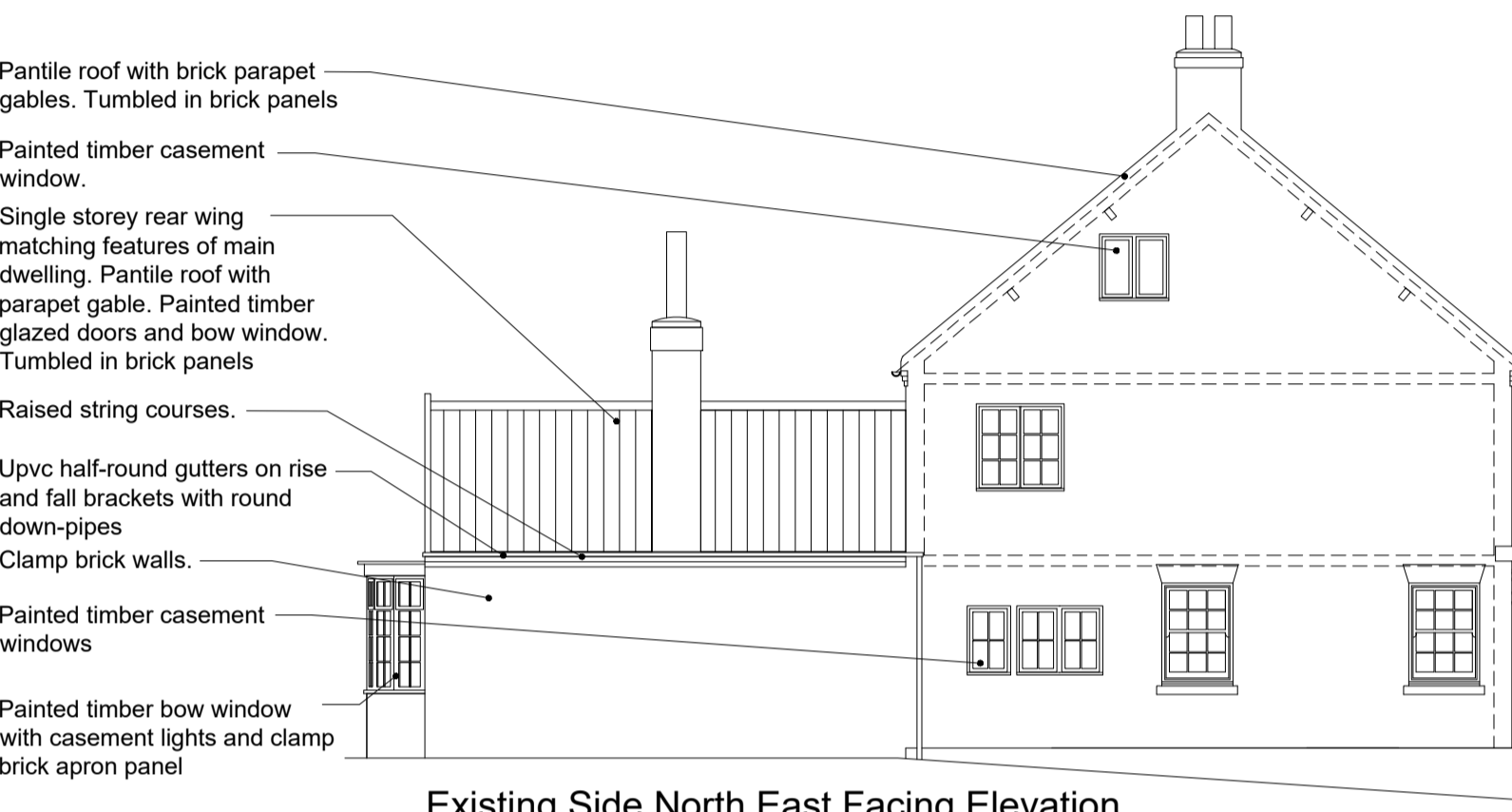
Existing Side North East Facing Elevation
