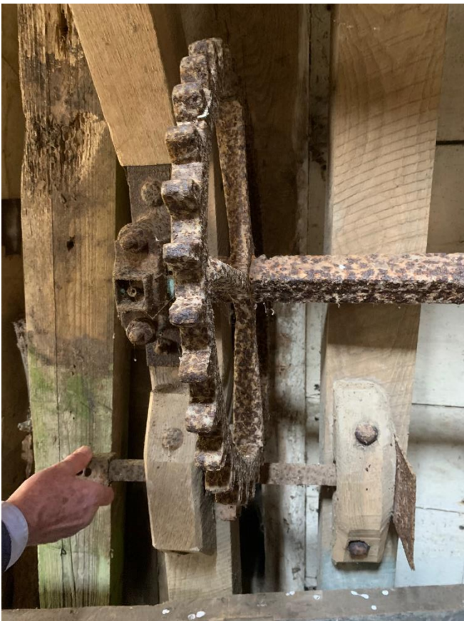
Ancillary drive- showing the millers hand engaging the drive. The ancillary drives were an important part of the mechanism to operate the sack hoist, pulling sacks from the spout floor (ground floor) to the bin floor (the second floor)
