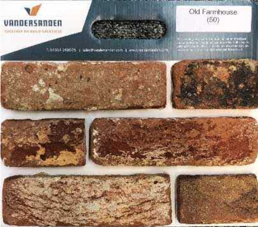
Photo 2.2 –Sample of Vandersanden, Old Farmhouse, note samples in photos are manufacturers standard sample boards showing the proposed bricks only (we will construct a sample panel on site with the proposed white cement at a later date)
