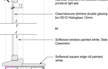
Spray foam to reveal of window to provide seal, to allow for differential movement.
