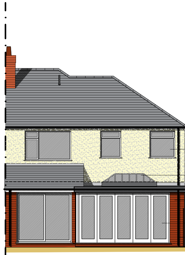
PROPOSED REAR ELEVATION scale 1:100
