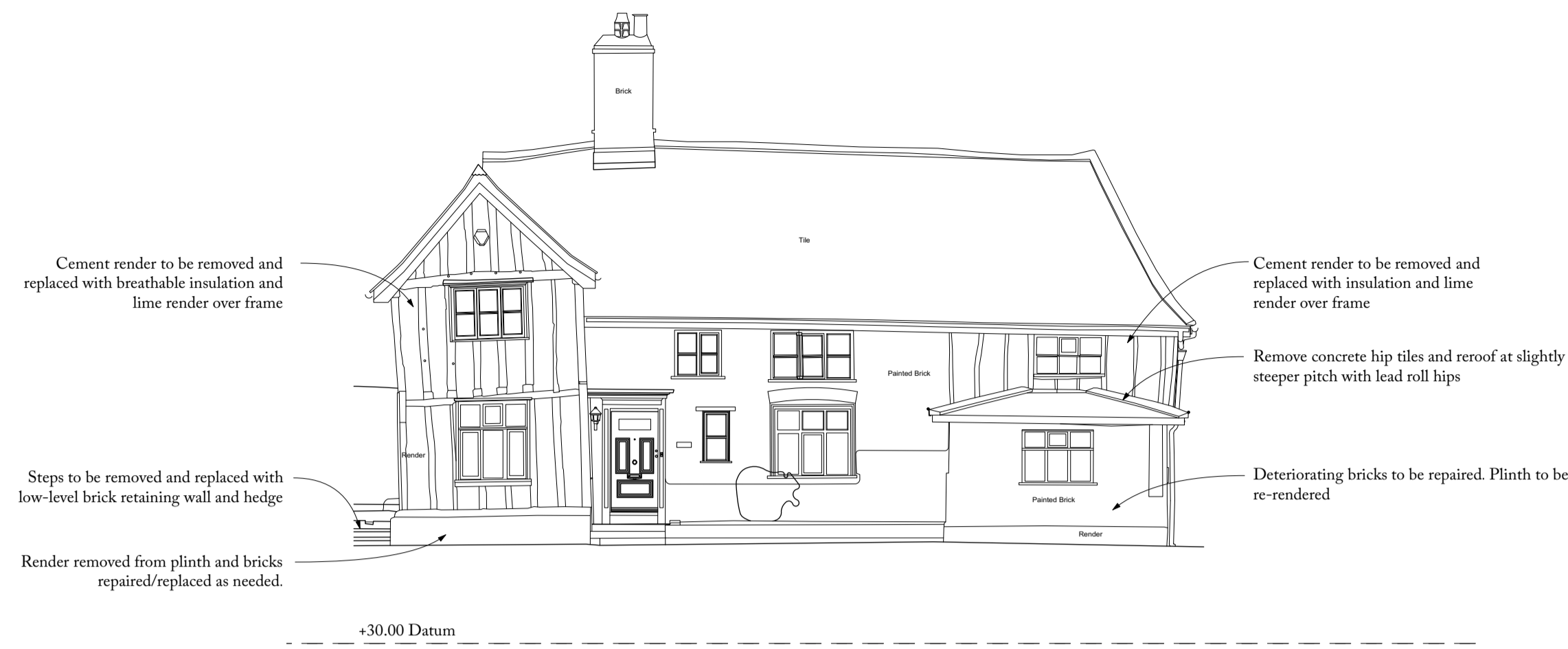
1 SOUTH ELEVATION As Existing, 1:100
