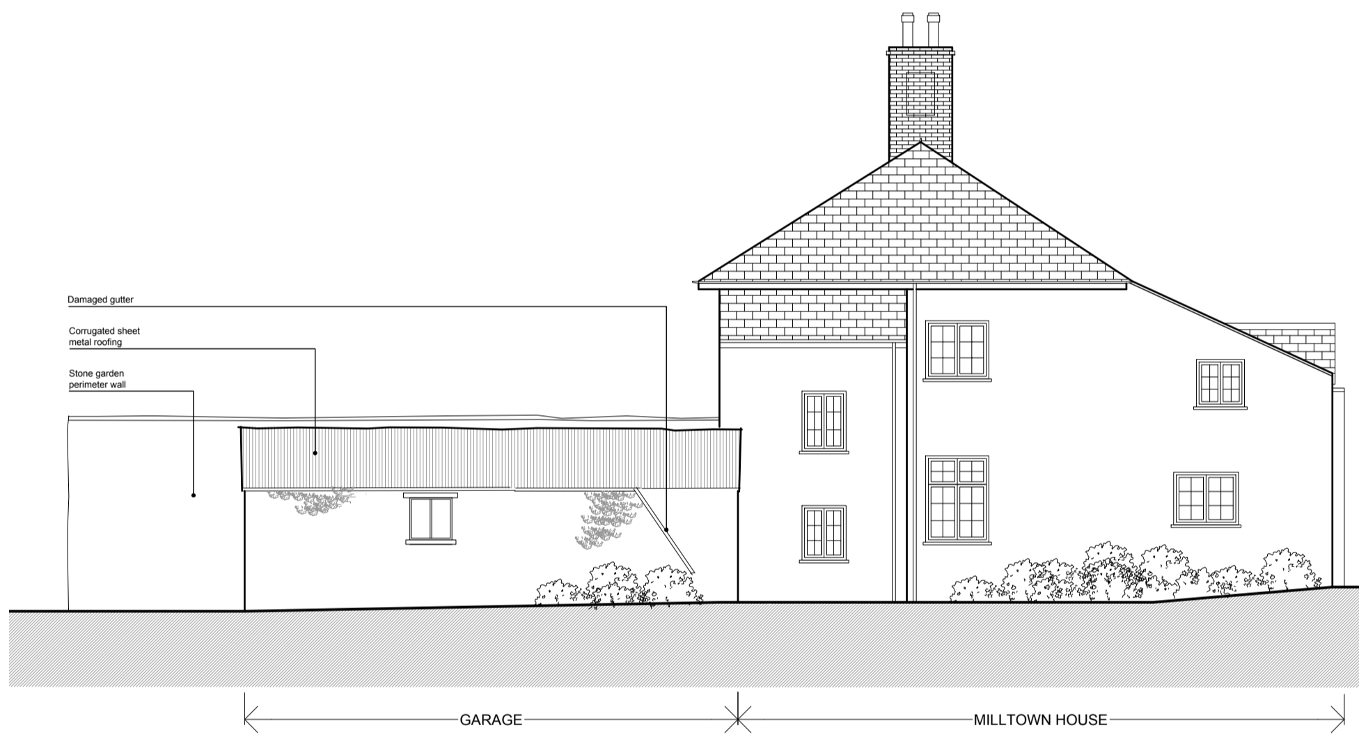
03 Existing East Elevation 1:100
