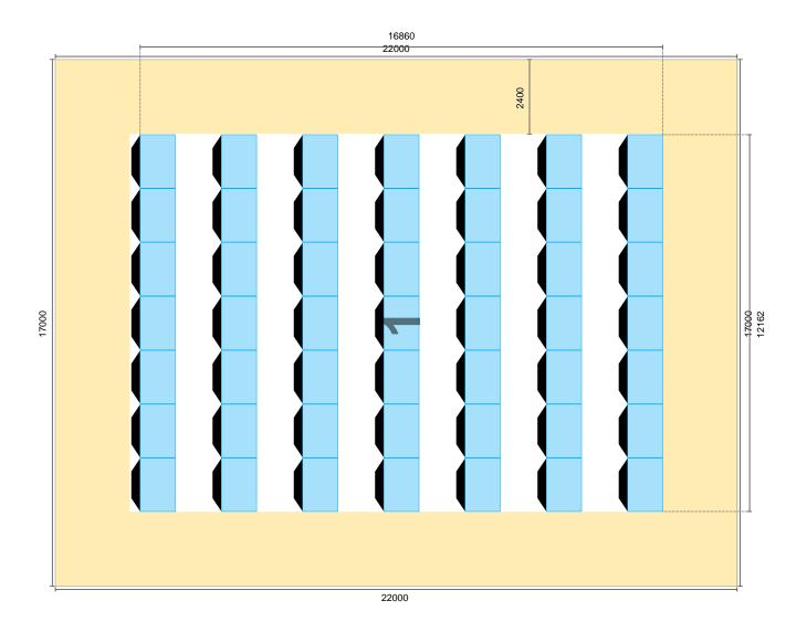
MODULE FIELDS \*Measurements in mm
