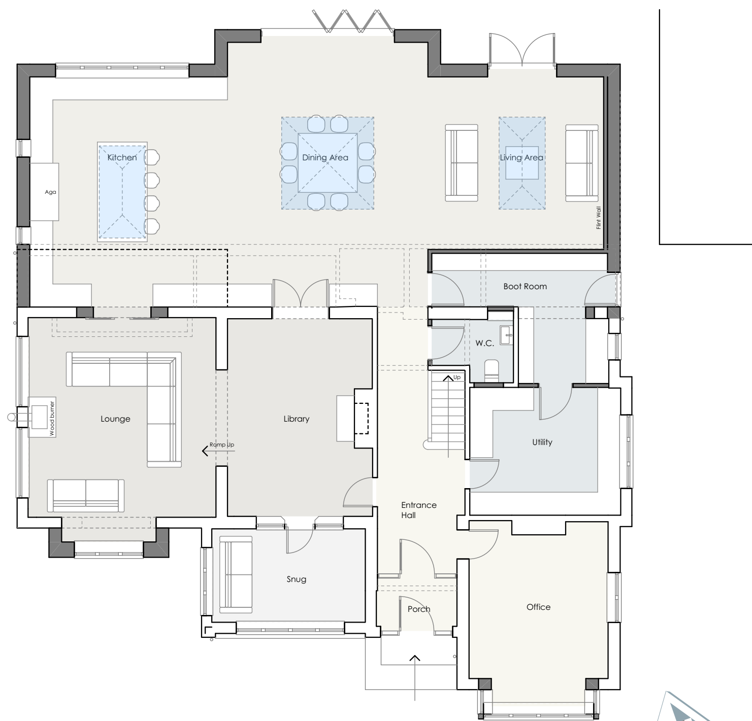
GROUND FLOOR PLAN Scale 1:100
