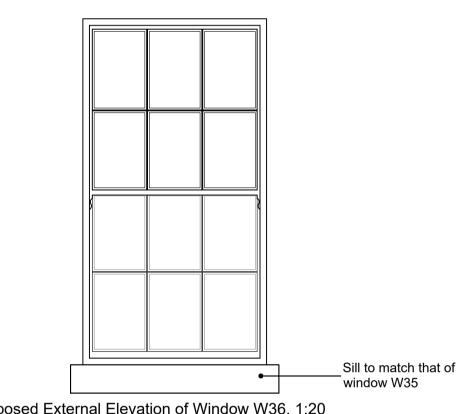
Proposed External Elevation of Window W36, 1:20
