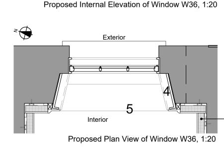
Proposed insulation to be approved through discharge of condition 11 of Listed **Building Consent** 20/01316/LBC
