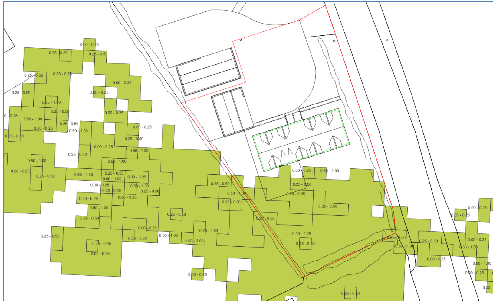
1000-Year Surface Water Flood Velocity
