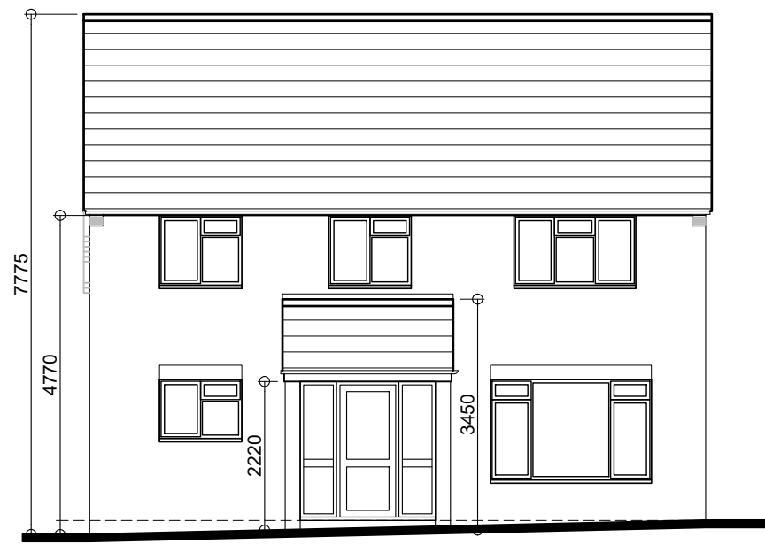
Existing Front Elevation Scale 1:100
