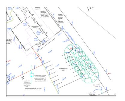
It is impractical to raise the ground floor levels by 1.4m to be above this level. It is therefore proposed to raise the ground floor levels by 600mm in line with standard EA guidance and propose flood avoidance measures as follows.
