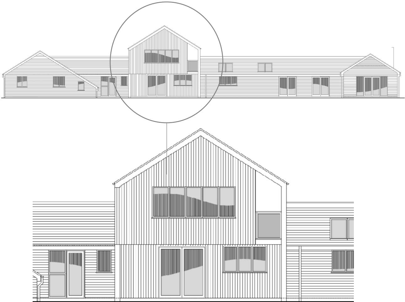
Figure 10: Proposed fenestration to First Floor extension
