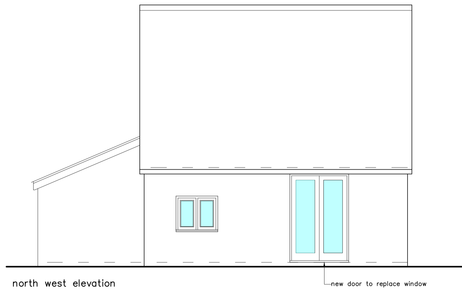
north west elevation
