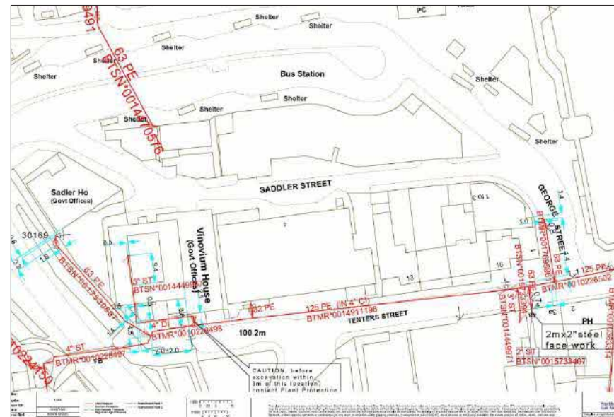
Fig. 32 Extract of Northern Gas Networks utilities information
