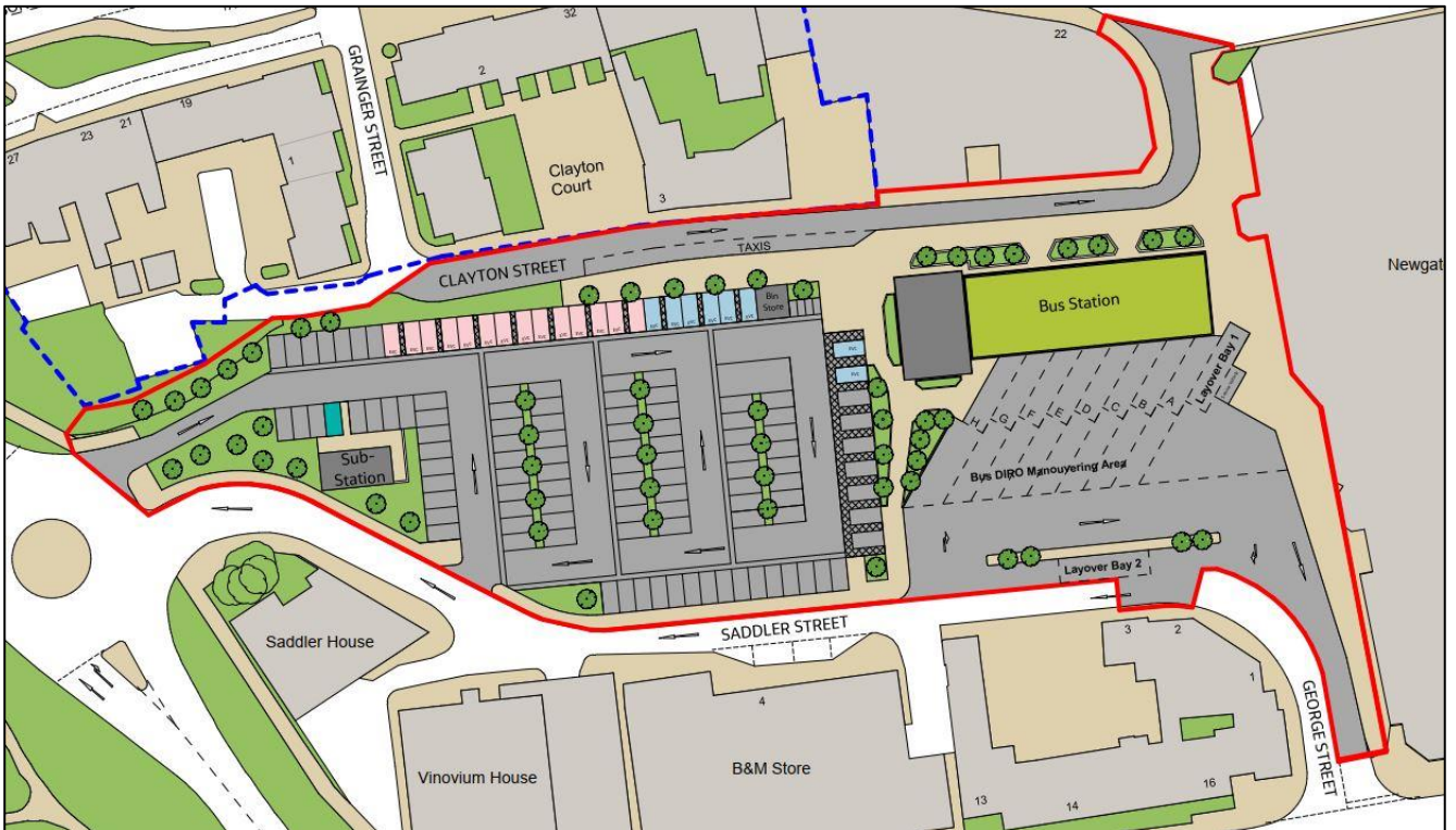
Figure 3.2: Proposed bus station design showing DIRO layout
