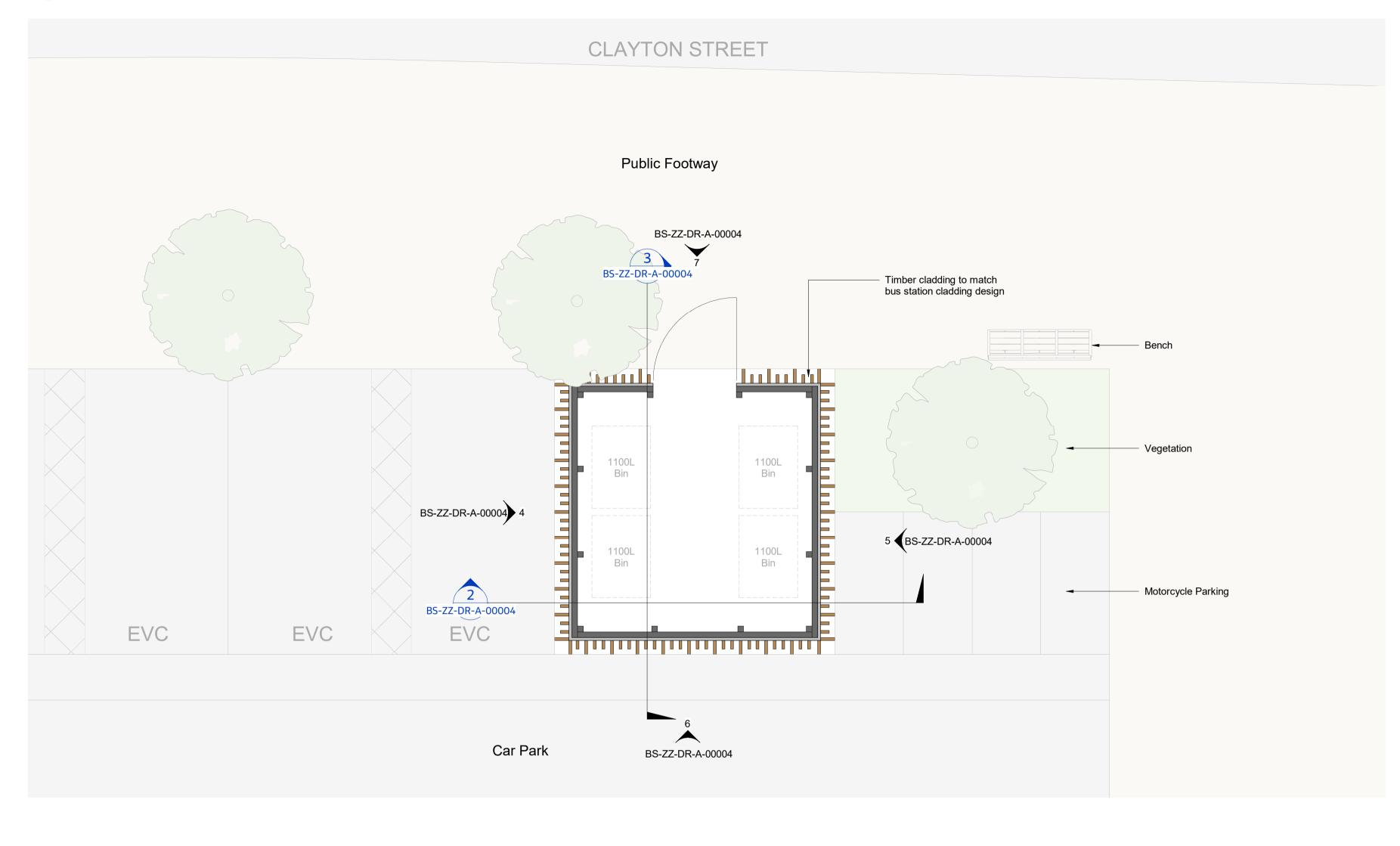
Timber fin cladding Post and horizontal rails for cladding 1100L 1100L support RC Slab
