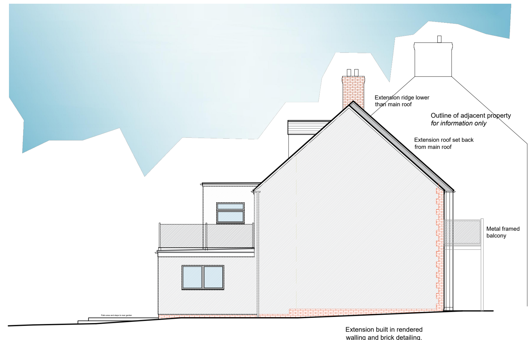
PROPOSED SOUTH WEST ELEVATION 1:100 SCALE
