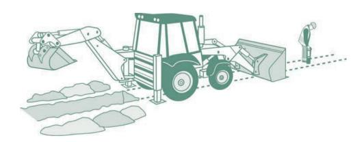
By hand, dig trial holes to locate the exact position of all cables.
