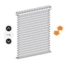
Use the  $\ensuremath{\mathsf{UP}}$  and / or  $\ensuremath{\mathsf{DOWN}}$  buttons to adjust the blind to the new lower stop position.
