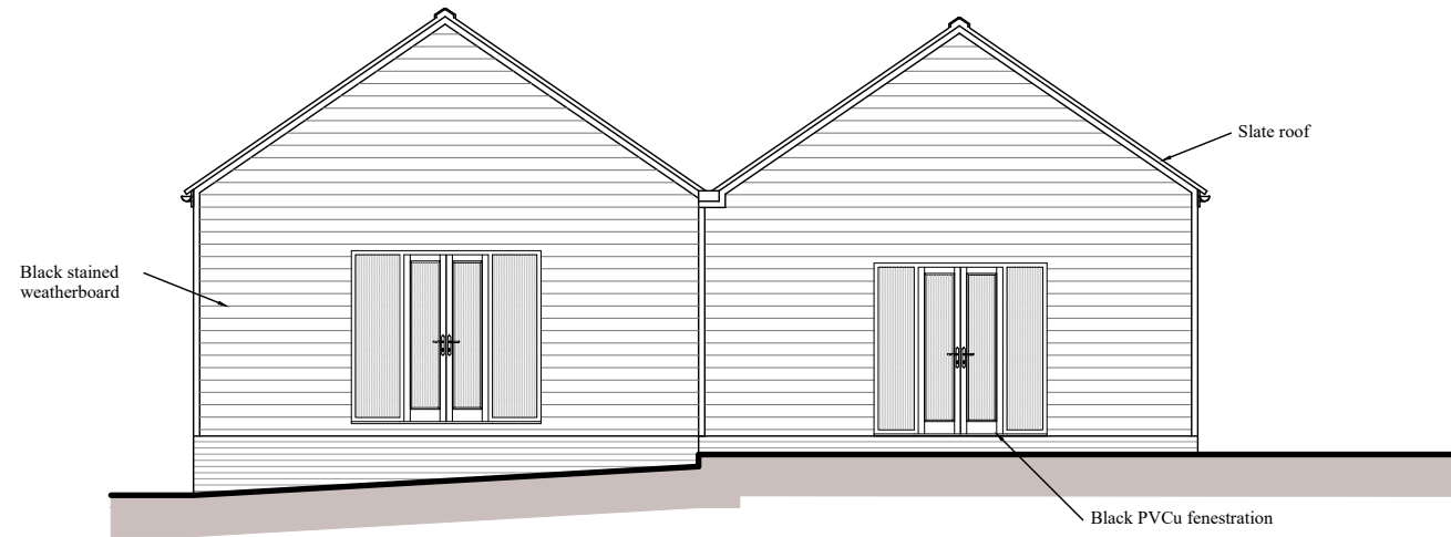
SOUTH WEST ELEVATION
