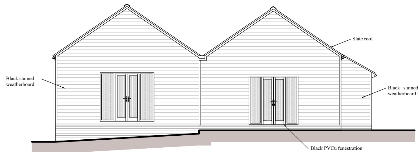
SOUTH WEST ELEVATION
