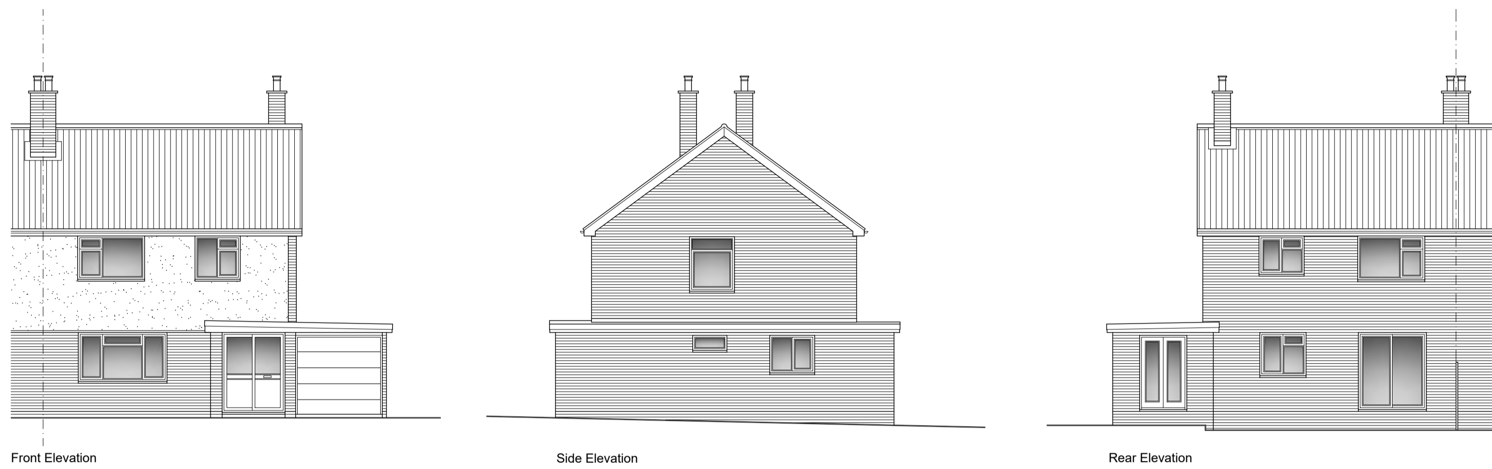
Front Elevation Existing Elevations Scale: 1:100
