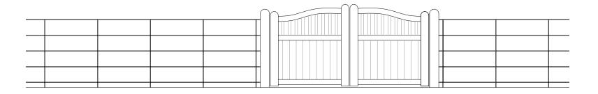
**Proposed Vehicle Gate & Estate Fencing** Elevation
