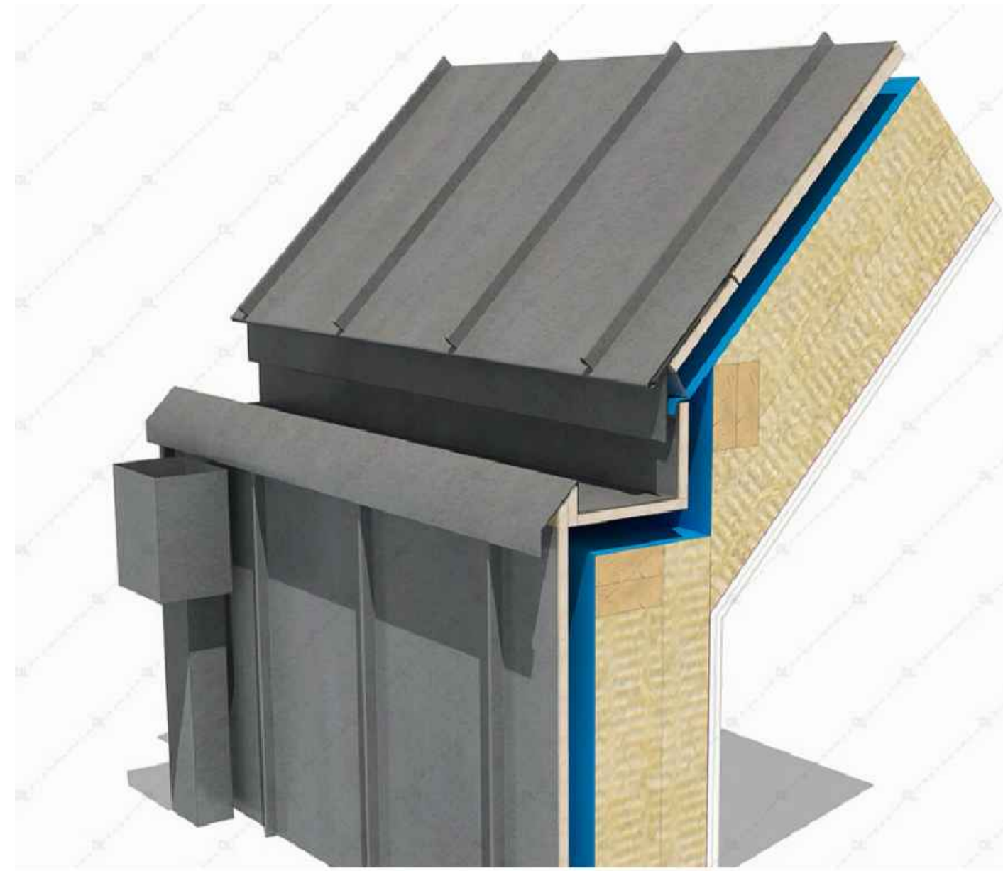
Kitchen extension eaves detail
