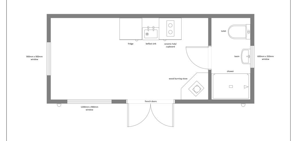
Shepherd's Hut Dimensions Length = 5382mm Width = 2200mm
