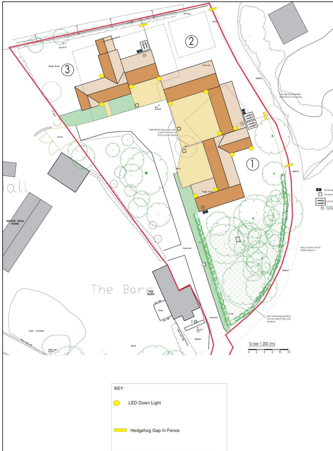
Figure 2: Recommended locations for lighting & hedgehog gaps.
